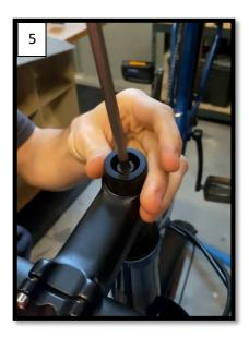
After that, screw the top cap until it makes contact (Figure 6). Then, loosen the stem bolts. Re-tighten the top cap bolt until there is no more play in the headset.
