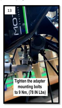
Spin the wheel to ensure it rotates freely. Remember to test the brakes to ensure they function correctly before using the bike.
