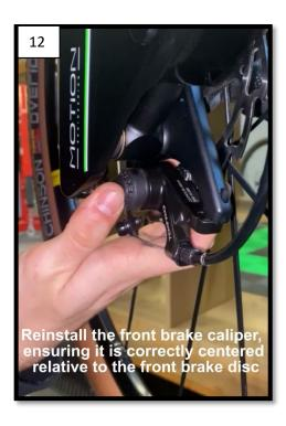
Using a torque wrench, tighten the brake caliper bolts to 9 Nm (78 in-lbs). Figure 13.
