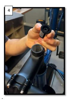
Use an Allen key to tighten the expander inside the fork steerer. (Figure 5).
